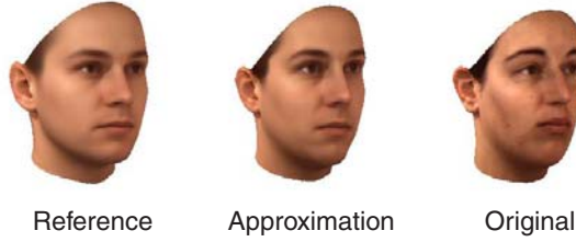
Fig. 10.4. Images of rendering of 3D lasers scans. The first is the reference with which correspondences are to be estimated. The second is the fitting of the original with a morphable model constructed with a subset of the scan for which correspondences were correct. The last one is the original scan.
