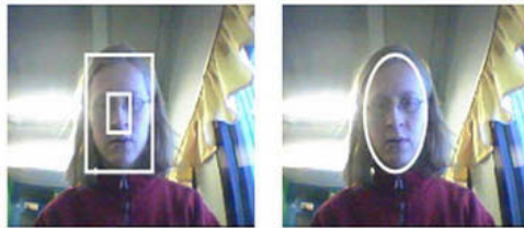
Fig. 6.5. The image on the left demonstrates the method suggested by Raja et al. [32]. The skin color model is updated by the area (inner box) calculated from the face localization (outer box). The elliptical constraint used to select pixels for adaptation by Yoo and Oh [51] is shown in the image on the right.
