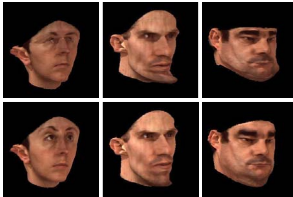
Fig. 10.3. Correspondence artifacts are visualized by making shape caricatures (i.e., extending the shape deviations from the average). Top row: Three caricatures yielded by the original morphable model are shown. Bottom row: Caricatures of the same scans obtained by the regularized morphable model are presented. Clearly, the bottom row is less perturbed by correspondence artifacts.
