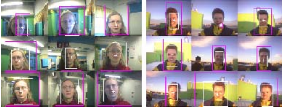
Fig. 6.12. The image on the left shows tracking results for an indoor movie and the one on the right for an outdoor movie. The skin locus approach was able to track despite widely varying illumination. (See insert for color reproduction of this figure)
