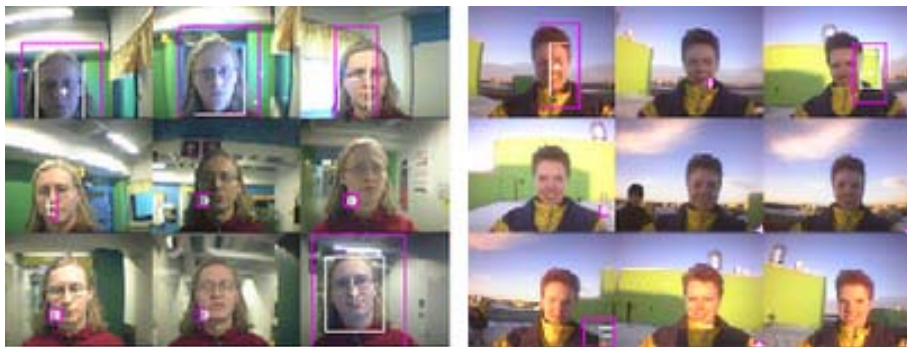
Fig. 6.13. The image on the left shows tracking with a fixed skin color model obtained from the first frame. This model is valid so long as the illumination variation is small. The right image displays adaptive tracking using the elliptical constraint suggested by Yoo and Oh. As can be observed from these images, this constraint is sensitive to the localization quality and may start to track other objects. (See insert for color reproduction of this figure)
