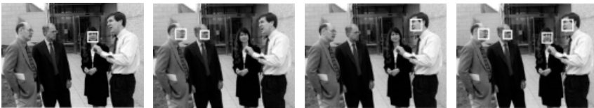
Fig. 2.14. Merging from different channels. From left to right: Outputs of frontal, left, and right view channels and the final result after the merge.
