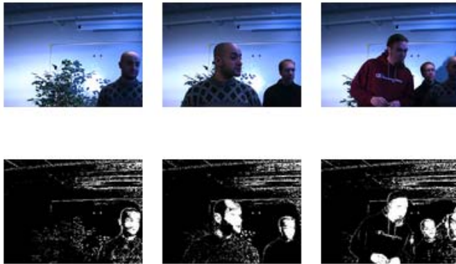
Fig. 6.10. A skin locus can be applied to images with one or more persons. The detection results are good for pure skin regions. (See insert for color reproduction of this figure)
